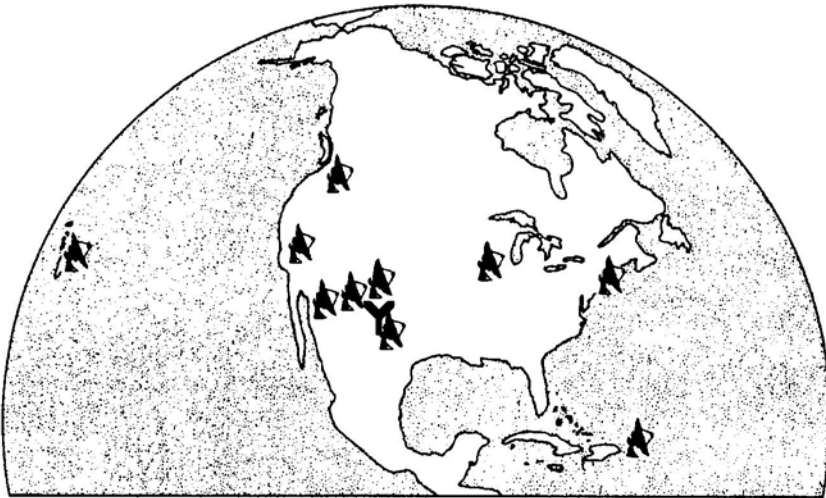
Figure 6. The distribution of the ten elements of the Very Long Baseline Array (VLBA). This network is often augmented with other radio telescopes such as the Very Large Array (a 27-element array operating as a phased array), shown here with the symbol Y, and the 100 m telescope of the Max Planck Institute for Radio Astronomy near Bonn, Germany.
